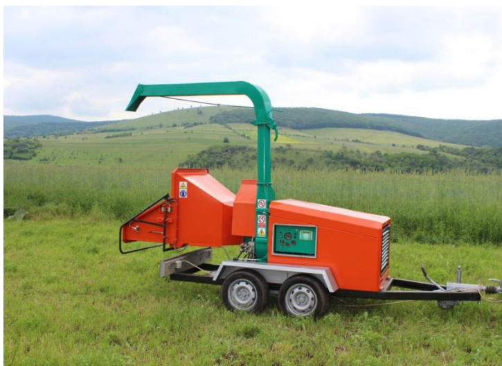
Figure 6 Mobile wood chipping unit (Erpék Ind SRL)
