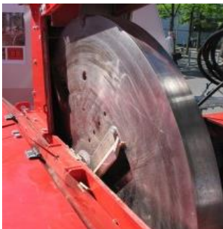
Flywheel with chipping knife of a disc-chipper ©greengain
