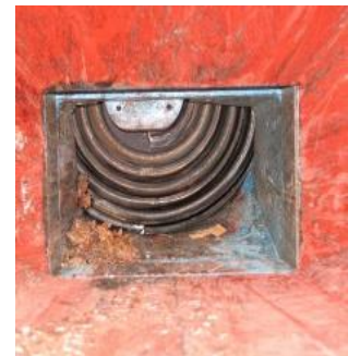
View into the grinding device of a screw-chipper ©greengain
