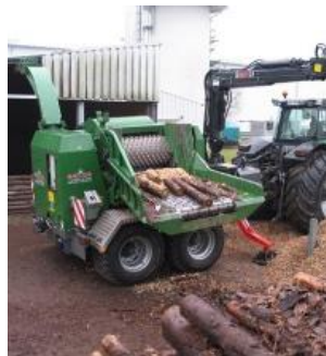
Drum-chipper with hydraulic forced infeed ©greengain
