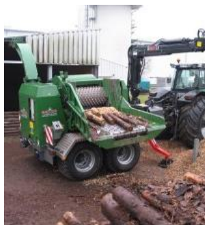
Drum-chipper with hydraulic forced infeed ©greengain
